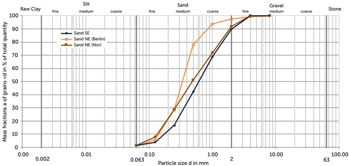
01 Comparison of the particle size distribution for the 0-2 mm fraction
