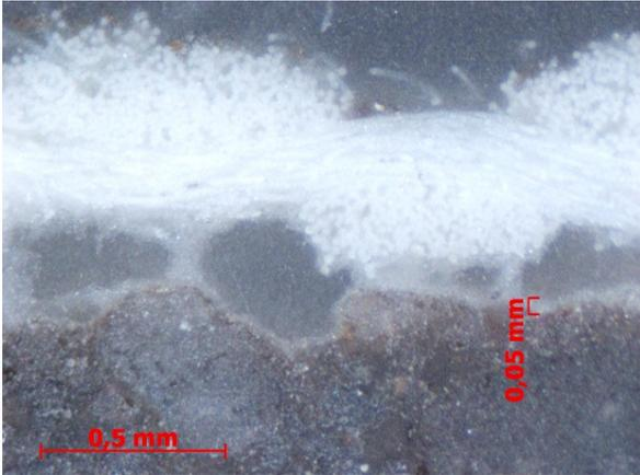
08 Polished section: Detail of the surface zone showing the textile wallpaper, paste a) and earth plaster mortar.
