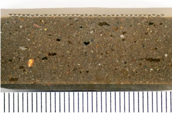
06 Polished section of a composite specimen of earth plaster, textile fabric, glued on flat with cellulose paste
