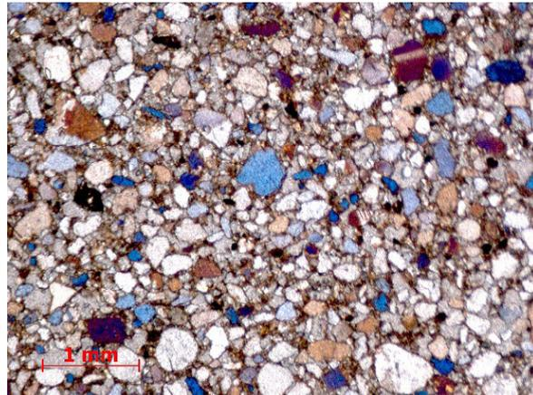
07 Thin section, 35 µm thick, showing parallel polarizers, a little binder (clay constituents), high quartz content and high open porosity
