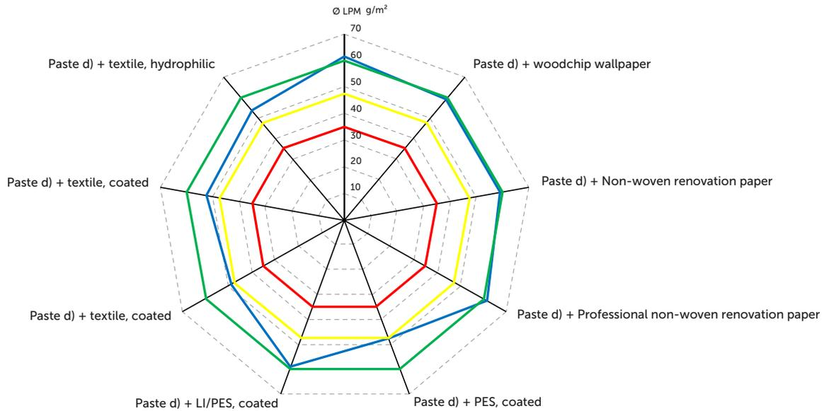
05 Comparison of the sorption activity (12-hour values) of untreated earth plaster mortars (above) with different application systems based on paste d)
