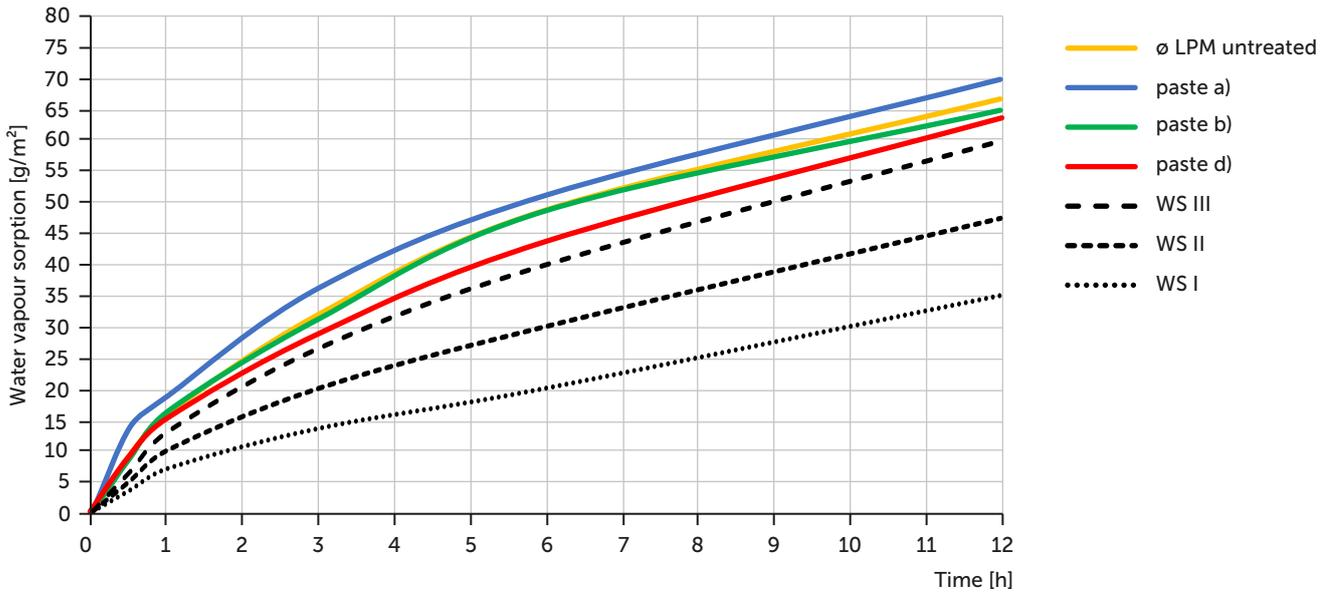
03 Water vapour sorption behaviour of the test surfaces with pre-glued and pasted (blue, green, red) test surfaces and the untreated (yellow) clay plaster mortar samples as well as the water vapour sorption classes WS I to WS III
