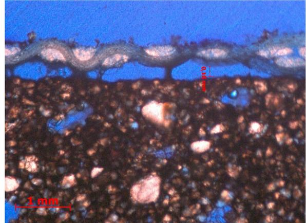
09 Thin section: Detail of the surface zone showing the textile wallpaper, paste d) and earth plaster mortar.
