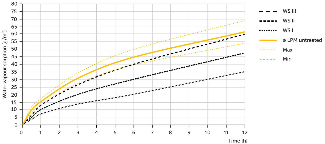
01 Water vapour sorption behaviour (mean value of 20 individual measurements) for untreated earth plaster mortar samples with minimum and maximum values (yellow) compared against the water vapour sorption classes WS I to WS III (black dashed lines)
