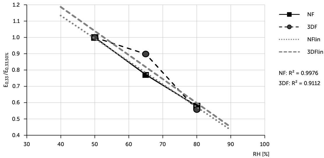
05 Related compressive strengths (left) and modulus of elasticity (right) of NF and 3DF blocks
