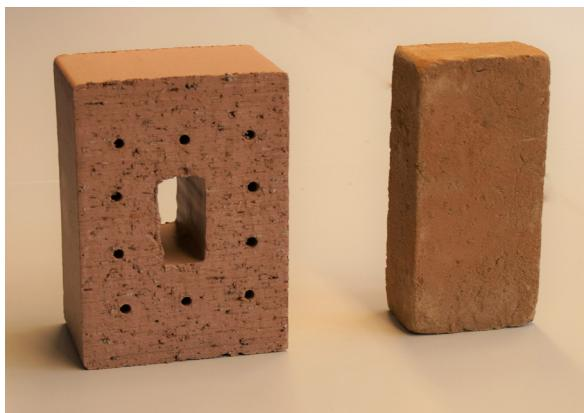
01 Extruded earth block 3DF (left), compression-molded earth block NF (right)
